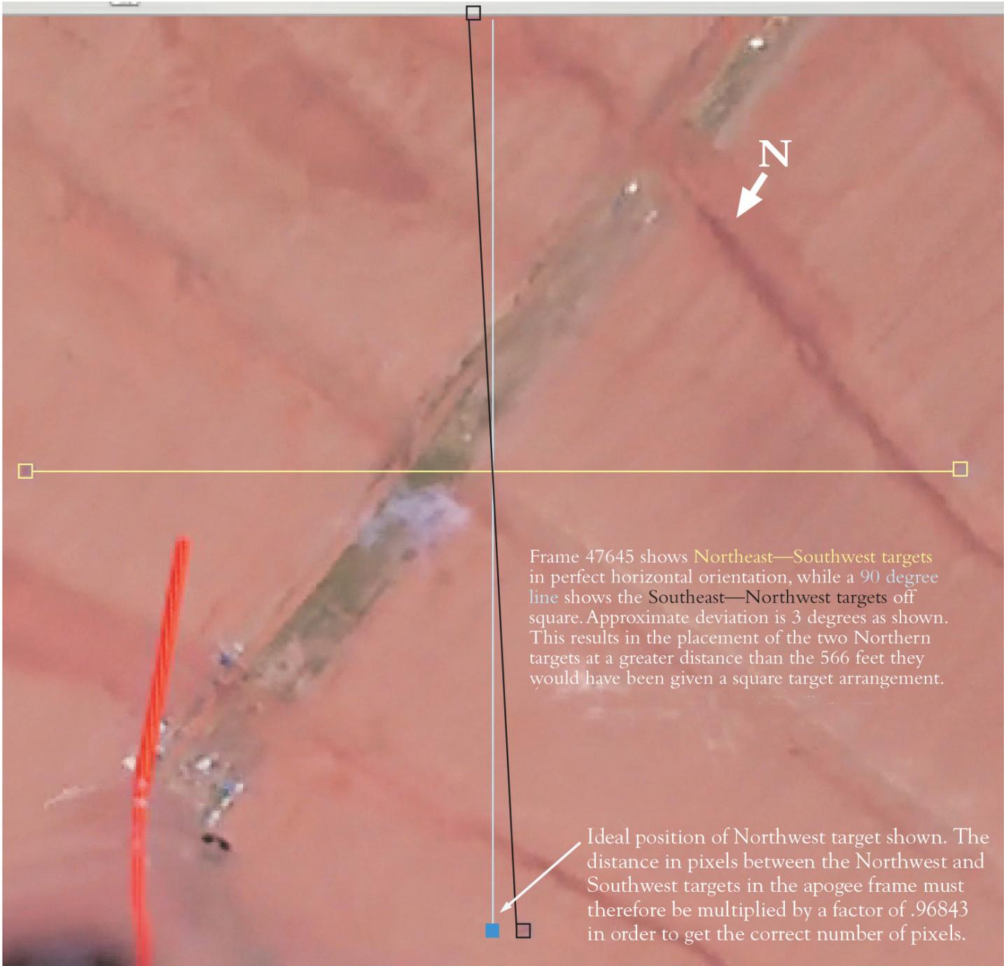
Frame 47645 shows Northeast—Southwest targets in perfect horizontal orientation, while a 90 degree line shows the Southeast—Northwest targets off square. Approximate deviation is 3 degrees as shown. This results in the placement of the two Northern targets at a greater distance than the 566 feet they would have been given a square target arrangement.
