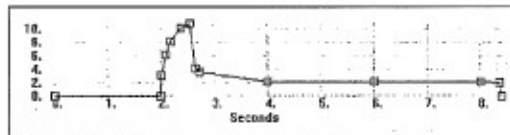
Simulation #6: The thrust curve of the delayed-start motor in Simulation #5 was created by shifting each of the data points over by two seconds in the motor wrasp data file. A program like Apogee Components' "EngEdit" is required to modify thrust curves like this.
